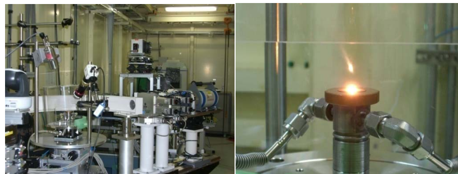
Aerodynamic levitation furnace at SPring-8 BL04B2 for in-situ XRD
