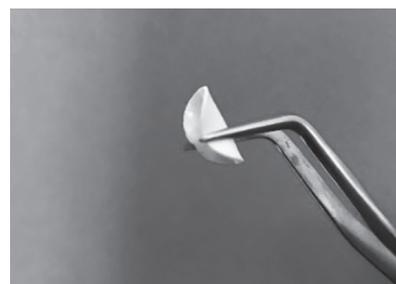
Fig. 1. Appearance of polyether/LLZO composite electrolyte ( $x = 1$ ).
