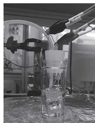
Figure 1 Photograph of Ni deposition on Cu foils.
